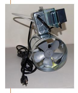
9000-Auto and 9008 Auto Duct Fans are controlled by an Air Pressure Sensing Switch. The Air flow in the duct turns the fan on and off. The switch is factory mounted and wired with a 10 foot line cord.
